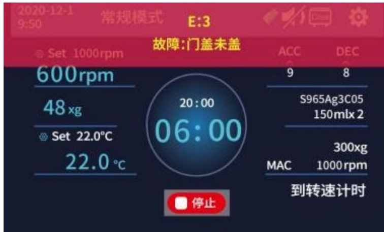
Figure 4-2. General centrifugal fault alarm example interface
